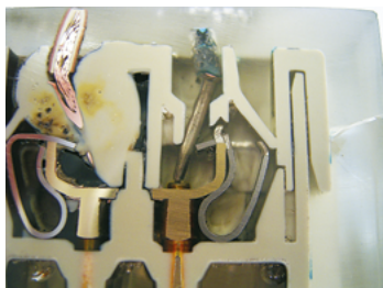
Figure VI-7: The consequences of improper assembly (shown here on the Han® ES), close-up
