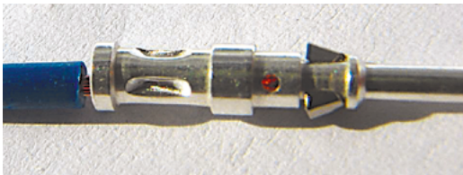
Figure V-12: Turned Han D® contact - proper stripping (depth + length) - inspection hole filled - crimping is uniformly central
