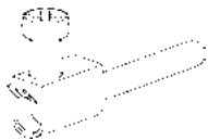
Figure III-4: Screw terminal with wire protection
