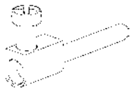
Figure III-5: Screw terminal without wire protection
