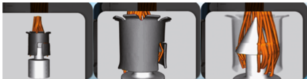
Figure VII-5: X-ray images of Han-Quick Lock®
