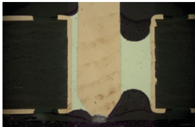
Figure VIII-11: Soldered joint with borderline degree of filling
